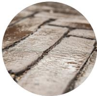
Vande Moortel clay pavers are ideal for the construction of water-permeable paving due to their specific natural character and quality characteristics. In conjunction with the correct joint filling, our moulded clay pavers provide enough space for rainwater to infiltrate the subsoil via the traditional natural joints between the clay pavers. Unlike extruded pavers or concrete pavers, with Vande Moortel clay pavers you are therefore not obliged to work with spacers.
