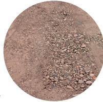
For effective compaction, a fraction of 0/32 with continuous grain distribution is recommended.
